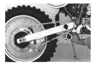
**CAUTION:** When mounting the chain masterlink clip, the closed side of the masterlink clip must point in running direction.
