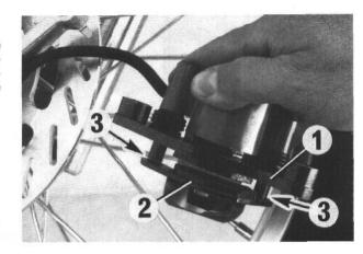
Remove the second brake pad (4) from the brake caliper carrier. Clean the brake caliper and brake caliper carrier with compressed air, check the rubber sleeve on the guide bolts for damage and grease the guide bolts if necessary. Install new brake pads in the opposite order and screw the brake caliper carrier tight.
