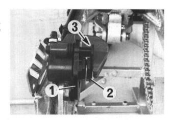
Remove the second brake pad (4) from the brake caliper carrier. Clean the brake caliper and brake caliper carrier with compressed air, check the rubber sleeves on the guide pins for damage and lubricate the guide pins if necessary. Install new brake pads.
