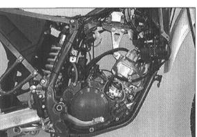
Remove engine screws, engine-retaining panels and swingarm pivot. Heave engine to the right out of the frame.
