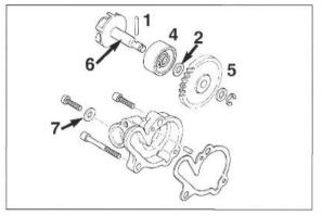
SHAFT SEAL RING **4**Check it for damage and tightness.
