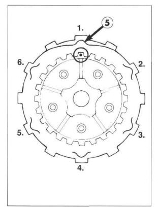
Each of the noses 9 of the following steel disks must be turned clockwise by 60° as compared to the previous one (see drawing).
