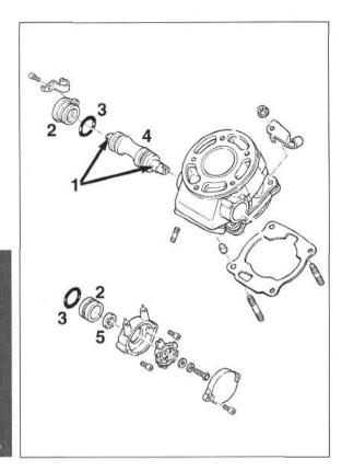
Clean all exhaust control components and check them for wear and damage.
