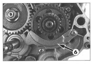
Apply Loctite 242 on two screws and mount the guide piece 6.
