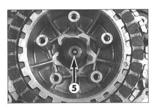
Insert push rod and ball 6 into main shaft.
