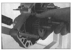
Use a plastic hammer to tap lightly on the countershaft and remove both transmission shafts.
