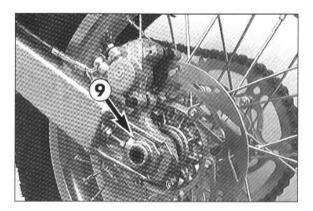
The rear wheel is remounted in reverse order. Before tightening the collar nut to 100 Nm (74 ft.lb), push the rear wheel forwards so that the chain tensioners lie on the tension screws.
