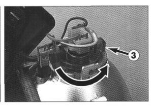
To change the headlight bulb, pull the plug from the bulb, turn the retaining clip counter clockwise, remove the bulb and dispose of the old bulb. Install the new bulb by aligning the light bulb pins with the socket groove . Attach the retaining clip and plug. Start the motorcycle and check the headlight for proper operation.
