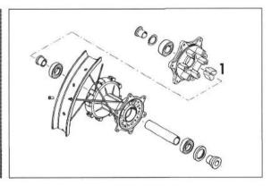
For this purpose, lie the rear wheel on a work bench with the sprocket facing upwards, and place the sprocket carrier into the hub. Now hold the rear wheel firmly and try to turn the sprocket. The sprocket may not turn more than a maximum of 5 mm (0,2 in) measured from the outside edge of sprocket. If freeplay in the sprocket is greater, all 6 cush-drive rubbers are to be replaced. Check the cush-drive rubbers for signs of damage and contamination. CAUTION
