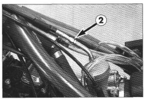
To adjust, remove the seat and the gastank, push the protective cover upwards, loosen the counter nut and turn the adjustment screw 2 accordingly. Turn the adjustment screw clockwise for more play or counterclockwise for less play. Tighten the counter nut, replace the protective covers and mount the gas-tank and the seat.
