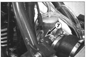
To adjust, remove the seat and the gastank, push the protective cover upwards, loosen the counter nut and turn the adjustment screw accordingly. Turn the adjustment screw clockwise for more play or anticlockwise for less play. Tighten the counter nut, replace the protective cover and mount the gas-tank and
