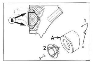
Mount the air filter on the filter support ②. Grease the front side ③ of the filter, to improve the seal. Mount the air filter and the filter support in the filter box. Make sure they are centered ③, and lock into place with the filter holder ①.
