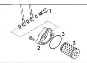
The O-ring 10 need not be replaced unless it is damaged. Press the O-ring into the groove of the oil filter cover, mount a new oil filter 10 on the oil filter cap and mount the unit. Insert the 3 screws and tighten them with 5 Nm (4 ft.lb). Mount the banjo bolt with the gaskets and tighten it with 15 Nm (11 ft.lb). Then start the engine and check the oil system for leaks.
