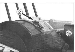
Insert the rubber ② into the opening of the housing and fasten the ignition cover with the two retaining springs.
