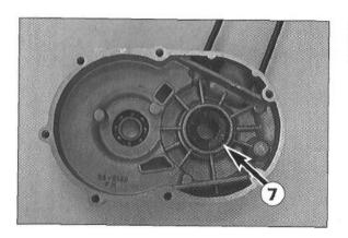
Shaft seal RING of the Crankshaft  $\odot$  Insert a new shaft seal ring from outside, the sealing lip facing inwards. The seal ring must be 2 mm (0.08 in.) below the edge of the housing.
