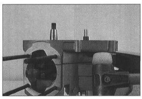
Lightly tap the right housing half with a rubber hammer until the housing half can be removed.
