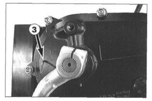
Unhook the kickstarter spring  $\ensuremath{\mathfrak{G}}$  and pull the kickstarter off the kickstarter shaft.
