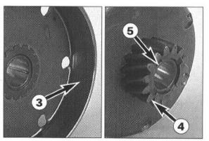
Check the running surface 3 of the clutch drum for grooves and signs of wear.
