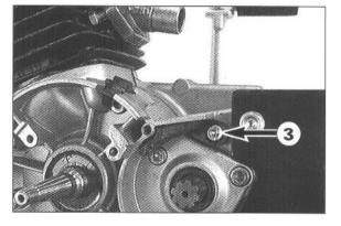
Remove screw 3 and take off the chain securing guide.
